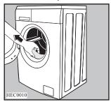
7. Fill the smaller upper hole and the two large ones with the corresponding plastic plug caps supplied in the bag containing the instruction booklet.
